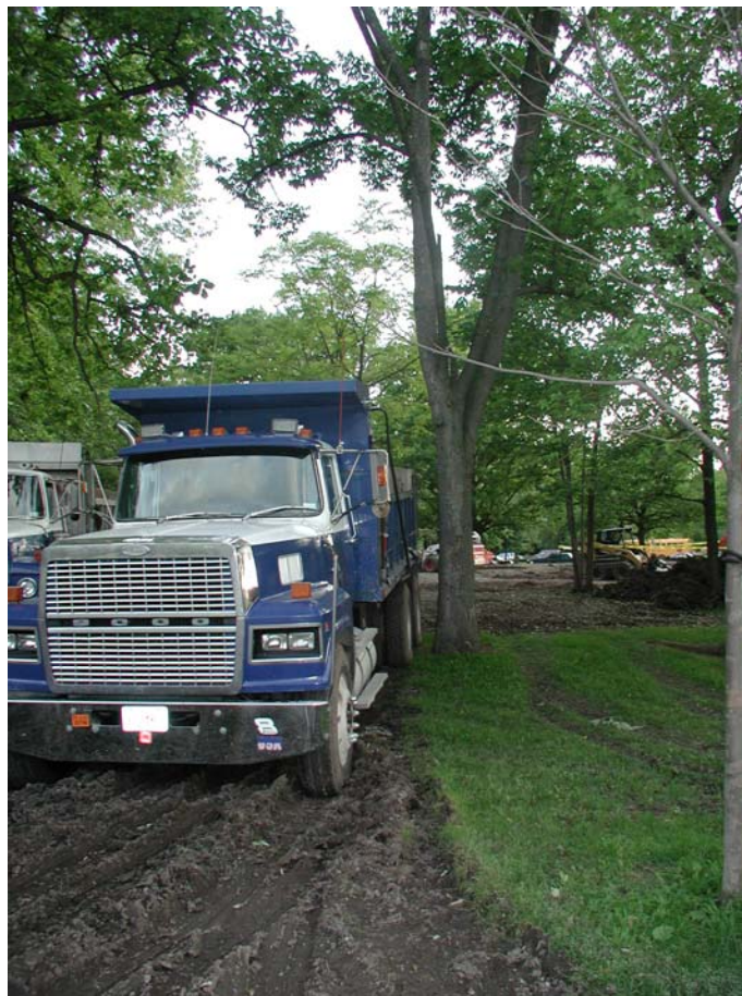
Figure 1. The weight from construction vehicles compacts and destroys urban soils – but does the vibration from these trucks affect soils nearby?
